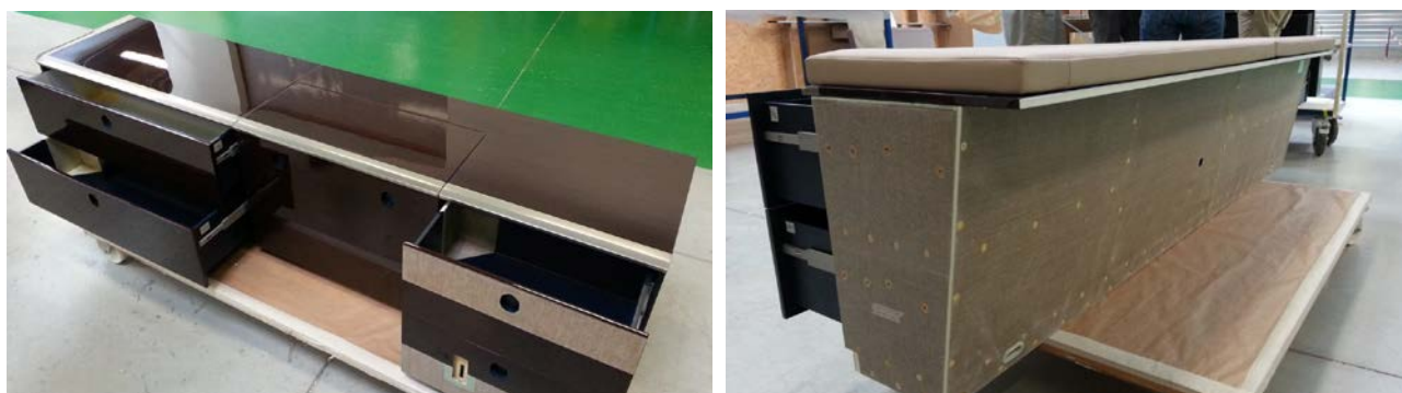
Figure 5.1.2 Aircraft cabinet prototype prepared by Dassault Aviation using GFTE bioepoxy sandwich composites
